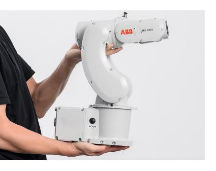
A small robot with a big performance designed to meet the trend towards the manufacture of miniaturized electronics and wearable devices. With the highest payload of 1.5kg, class-leading precision 0.01mm, and 30% smaller size, the IRB 1010 allows for the highest productivity and high-quality manufacturing.
